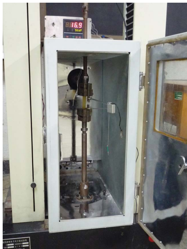
Figure 1 Thermomechanical testing device of SMPs. [Color figure can be viewed in the online issue, which is available at www.interscience.wiley.com .]
